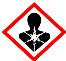
Serious Health Hazard
